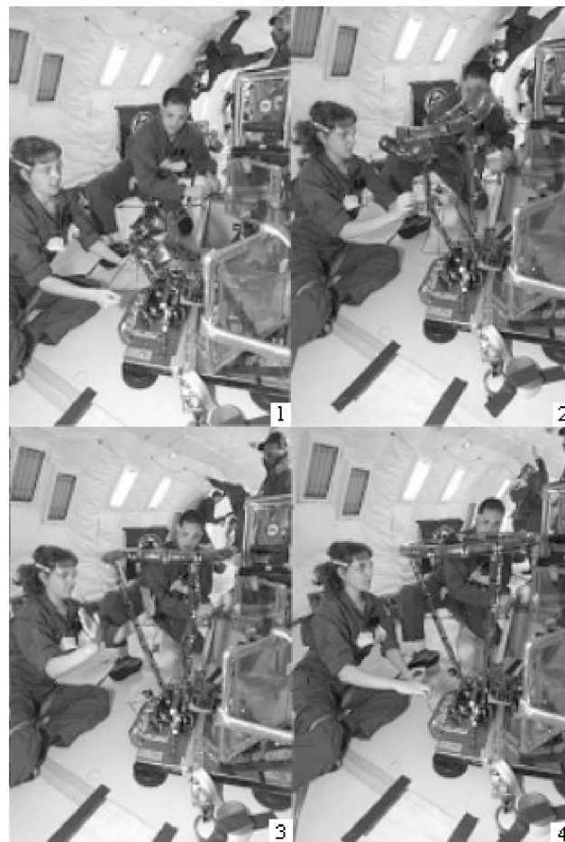
Fig. 5 Deployment sequence with staged release during pressurization.
